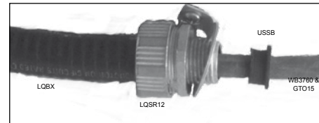
Figure 7 Slide USSB over WB3760 and GTO cable.. If necessary, Slide support ring over assembly and use metallic self tapping screw to hold assembly in place on wall or ceiling.
