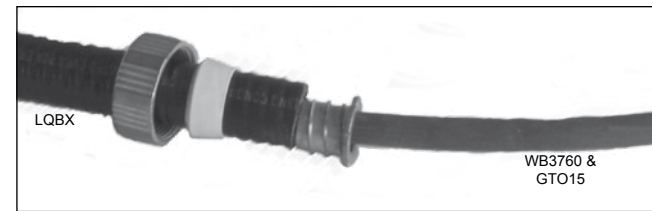
Figure 4 Slide the large metallic head over the LQBX/WB3760/GTO cable assembly, along with yellow plastic ring. Slide the 1/2" twist-on connector over WB3760 and GTO cable and screw it into the LQBX.
