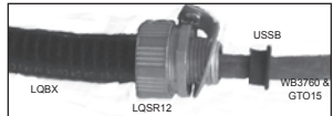
Figure 7 Slide USSB over WB3760 and GTO cable.. If necessary, Slide support ring over assembly and use metallic self tapping screw to hold assembly in place on wall or ceiling.
