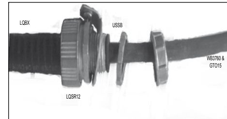
Figure 9 Slide locknut and metallic end bushing over WB3760 and GTO cable and screw all pieces together
