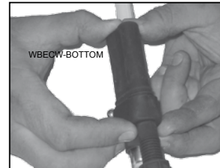
Fig.17 Placing your thumbs on the bottom part of the WBECW wetbits end cap wide, slightly push the cap forward into the top part until you hear the snap seal over the second rib of the cap
