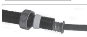
Figure 5 Slide the large metallic head over the LQBX/Integral Sleeve GTO wire assembly, along with yellow plastic ring. Slide the 1/2" twist-on connector over the integral sleeve and screw it into the LQBX.
