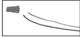
Fig. 6 When using USSB with standard sign ballast AWM 1015VW wire, there is no need of cutting the USSB. Simply use a drill of 5/32" maximum to perforate the second hole at bottom.
