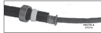
Figure 4 Slide the large metallic head over the LQBX/WB3760/GTO cable assembly, along with yellow plastic ring. Slide the 1/2" twist-on connector over WB3760 and GTO cable and screw it into the LQBX.
