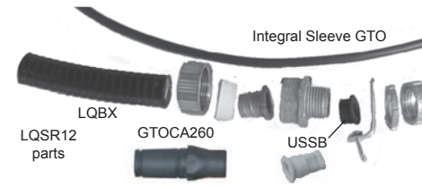
Fig.2 & 3 When using USSB with integral sleeve and GTO Cable Adaptor you must cut the USSB between the 2nd molded line delimitation to remove the three first sections of the bushing, keeping only the bottom part with the flanged collar. Make sure to grasp the flanged end of the USSB prior to cutting to reduce the likely hood that the piece you need to keep would fall to the ground.
