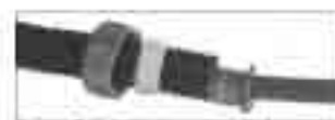
Figure 5 Slide the large metallic head over the LQSR/WB3760 sleeving GTO wire assembly, along with yellow plastic ring. Slide the 1/2" nut-on connector over the sleeving and cable assembly and screw it into the LQSR.
